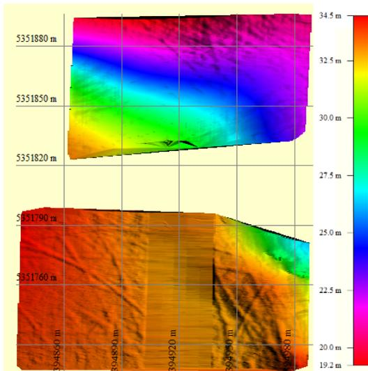
Fig. 2. Gridded Reson 7125 bathymetry on two parallel lines.
