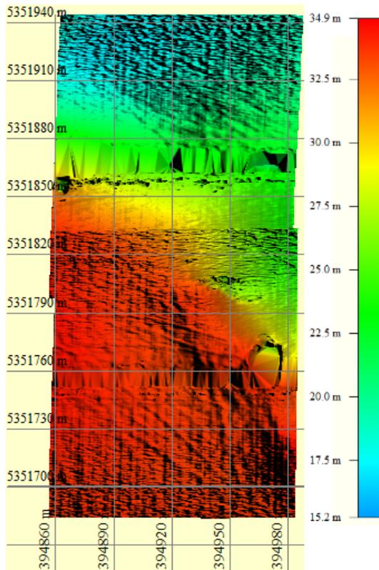
Fig. 1. Gridded Klein 5500 bathymetry on two parallel lines.
