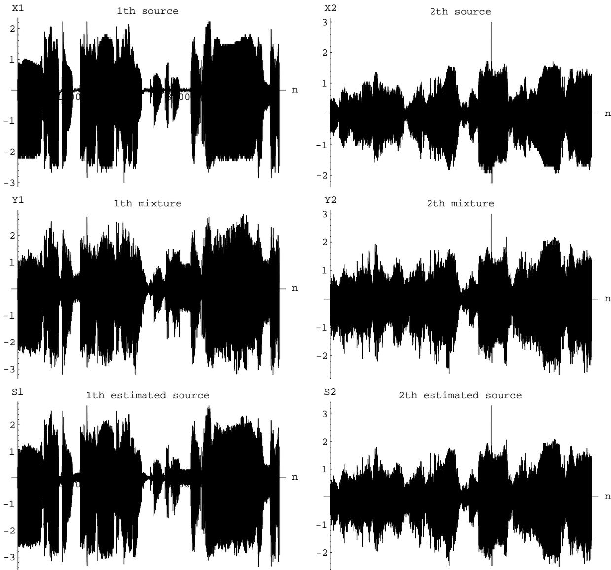
Figure 6: First column contains the signals of the first channel (i.e., first source, first mixture signal and the first estimated source), the second column contains the signals of the second channel.
