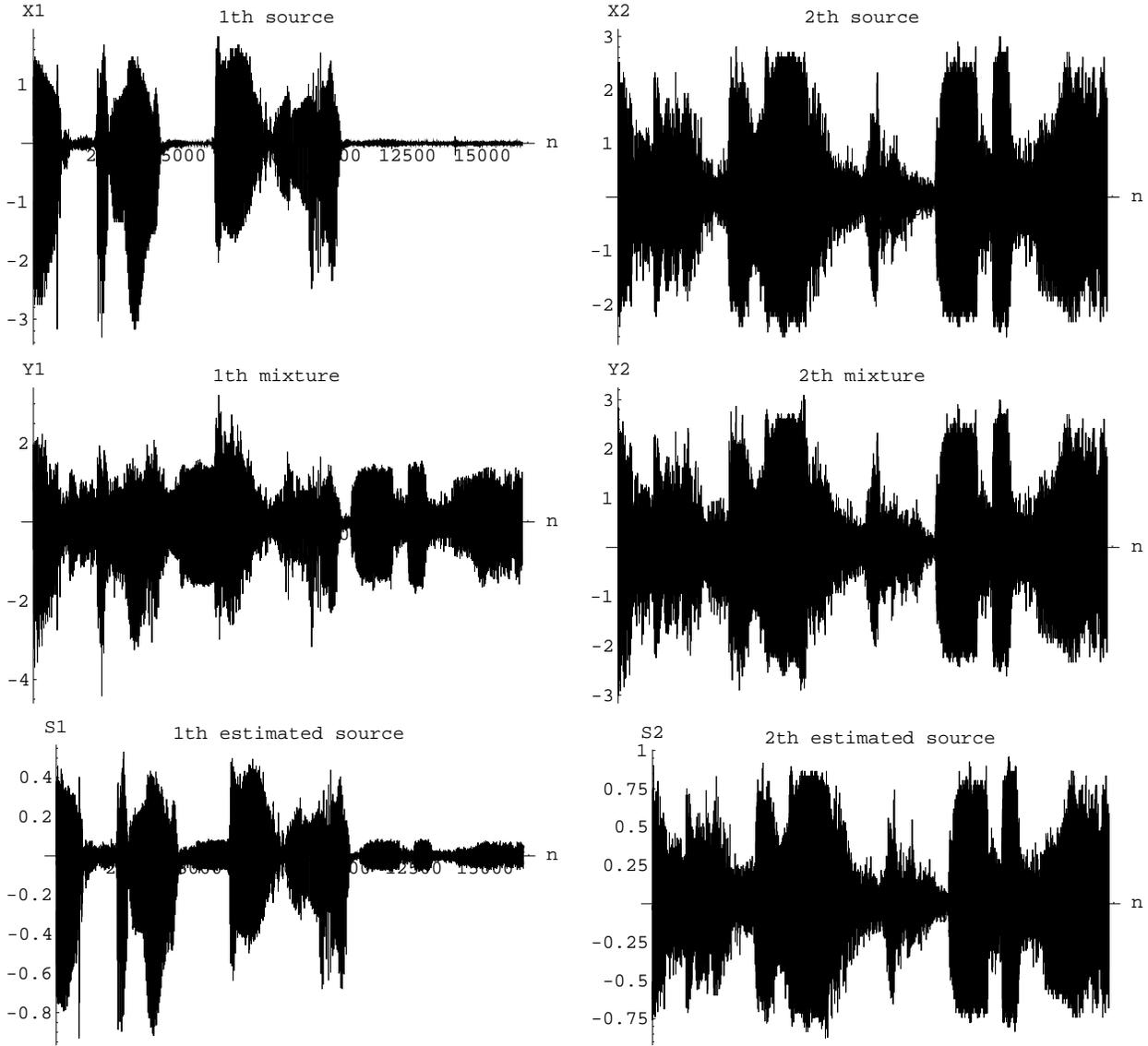
Figure 4: First column contains the signals of the first channel (i.e., first source, first mixture signal and the first estimated source), the second column contains the signals of the second channel.
