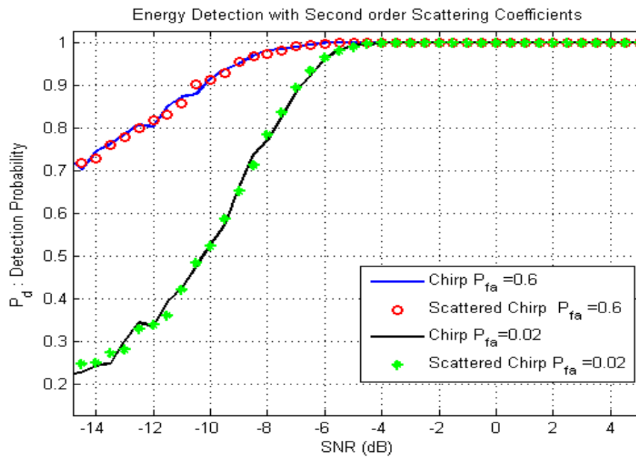
Figure 3. Detection probabilities vs. SNR for a chirp spread spectrum signal
