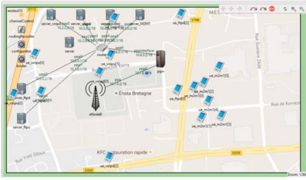
Fig. 5. Architecture with the SimuLTE modeler.
