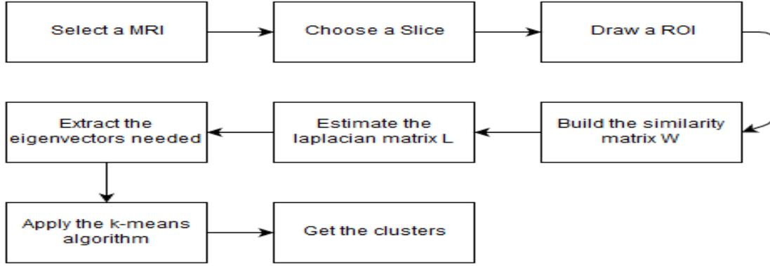
**Figure 2:** The proposed processing tool-chain.
