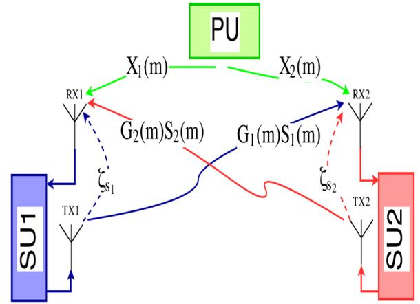
Fig. 2. The FDC-CR paradigm model: Two SUs are simultaneously transmitting and receiving at the same primary channel when detected as available
