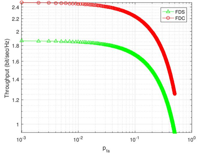
Fig. 4. The evolution of the channel throughput in terms of  $p_{fa}$  for  $p_d = 0.9$  and  $\sigma_w^2 = -100$  dB. SCS is adopted.  $\sigma_r^2$  and  $\sigma_p^2$  are fixed so that  $\Delta_{PU} = \Delta_{RSI} = 0$  dB. The power of the received  $SU$  signal is considered as:  $\Delta_{SU1} = \Delta_{SU2} = 5$  dB
