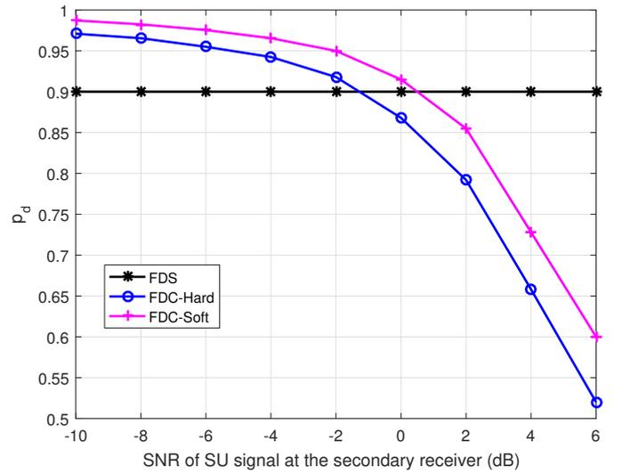
Fig. 5. The evolution of the probability of detection in terms of  $\Delta_{SU_i}$  for  $p_{fa} = 0.1$ ,  $\Delta_{RSI} = 0$  dB,  $\Delta_{PU} = -7$  dB and  $N=1000$  samples. The logic rule "Or" is used when hard combining scheme is adopted
