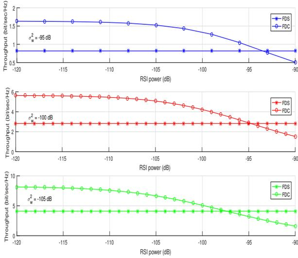
Fig. 3. Throughput of FDC-CR Vs. FDS-CR in terms of RSI power for several values of the noise power
